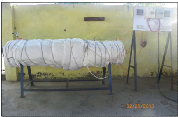
Fig.1. Experimental set-up of horizontal bio-char reactor System
