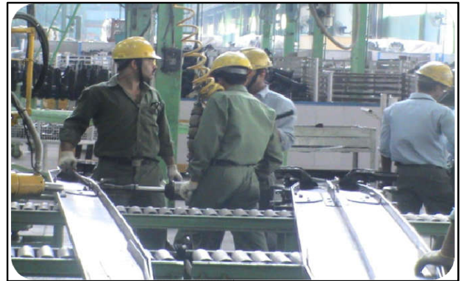
Fig. 2. Congested work space with limited access to the work piece. ‘Author’s work’
