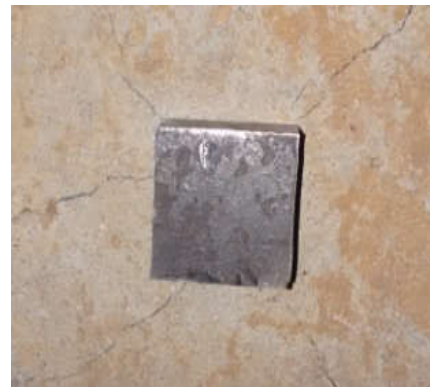
Fig 2(a): Tested cube for bearing area ratio 10
