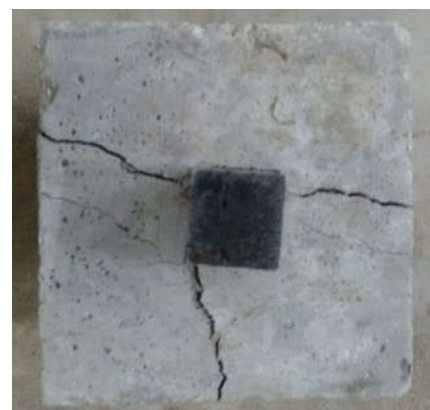
Fig 2(b): Tested cube for bearing area ratio 15
