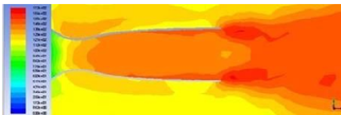
a. Base model of the CD nozzle
