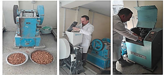
Plate 1. Sep's of crushing grounding the WCBs
