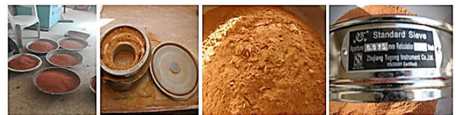
Plate 2. Step's of sieving and grains passing through 75µm
