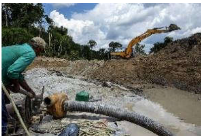
Figure 6. Illegal mining activity in indigenous lands in Das Tropas river, a tributary of Tapajós river, use of machines coupled to water hoses called "Tatuzão"
