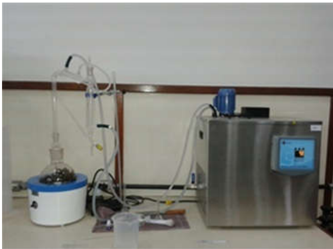
Figure 5. Essential oil extraction system. (a) Clevenger (b) Ultra thermostatic bath with pump
