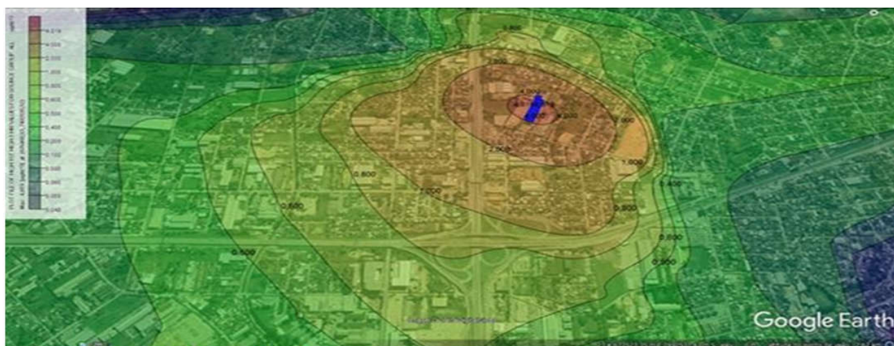
Figure 01. Modeling of PM10 with the AERMOD model - isolines of plume concentrations over inhabited areas, for a chimney with a height of 10 meters. Annual simulation
