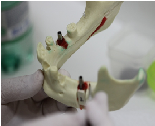
Figure 3. Test bodies positioned in the mandibles
