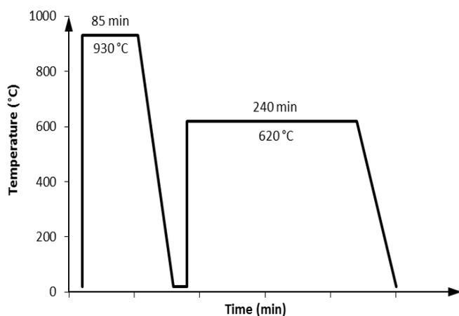
**Figure 1. Heat treatment cycle, composed by quenching and tempering, applied to the 13Cr supermartensitic stainless steel**
