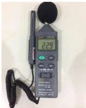
Figure 18. Istrutherm THDL - 400 Environment Meter thermohygrometer
