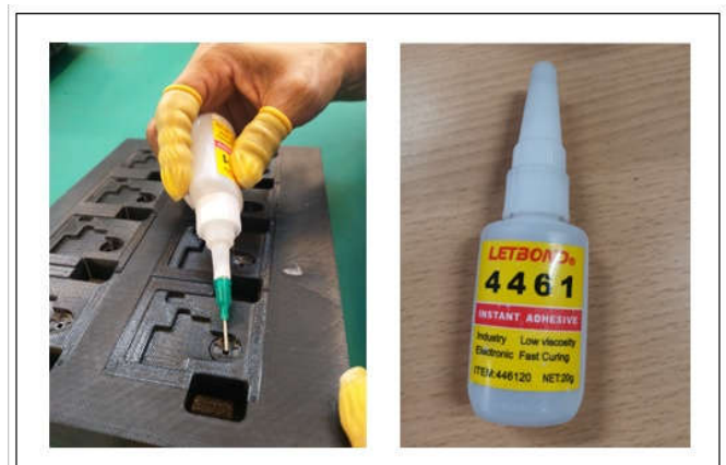
Figure 4. Adhesion process with Letbond 4461 glue Source: Authors, (2021)
