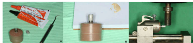
Figure 2. Temporary cement used (A); cemented crown (B) and illustration of mechanical cycling (C)
