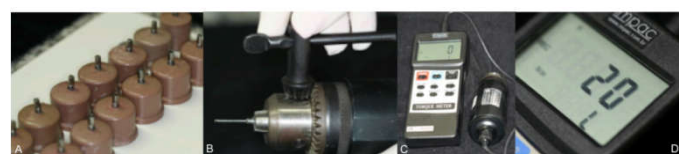
Figure 1. Embedded specimens with the trunnions in position (A); 1.17 key coupled to the digital torquemeter (B); digital torquemeter (C) and illustration of 20N.cm torque (D)
