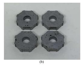
Figure 1. Cores of (a) stator and (b) rotor
