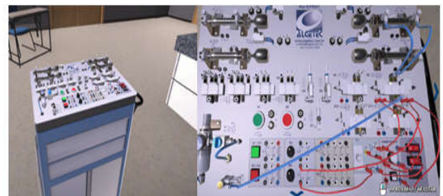
Figure 2. Bench for virtual experiments: a) virtual bench overview; b) view of the virtual assembly worktable
