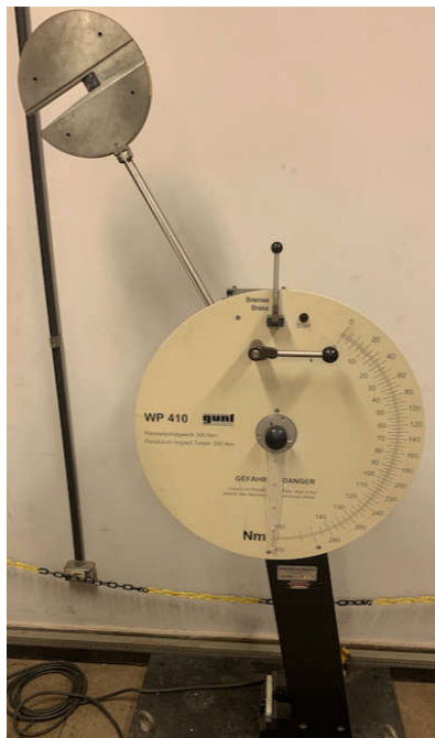
Fig.9 Impact machine used during the tests
