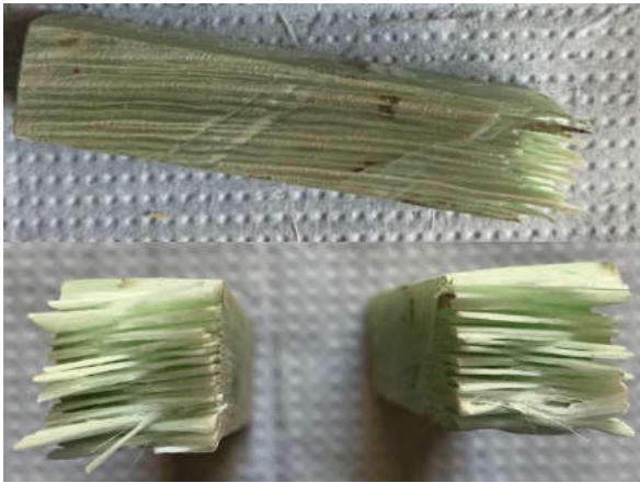
Fig.7 Specimens #5 of glass fiber after Charpy test
