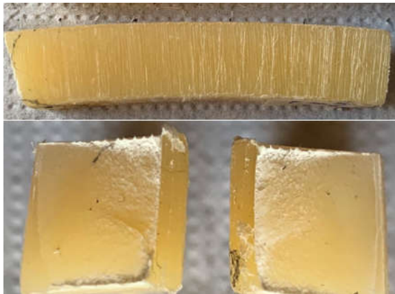
Fig. 8. Specimens #1 of PEHD after Charpy test
