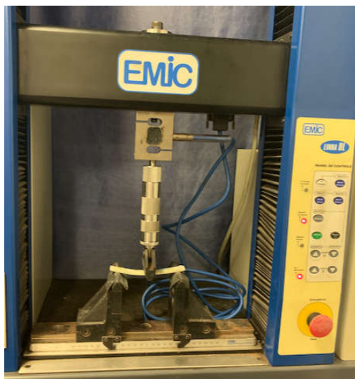
Fig.15 Flexural machine used during the tests
