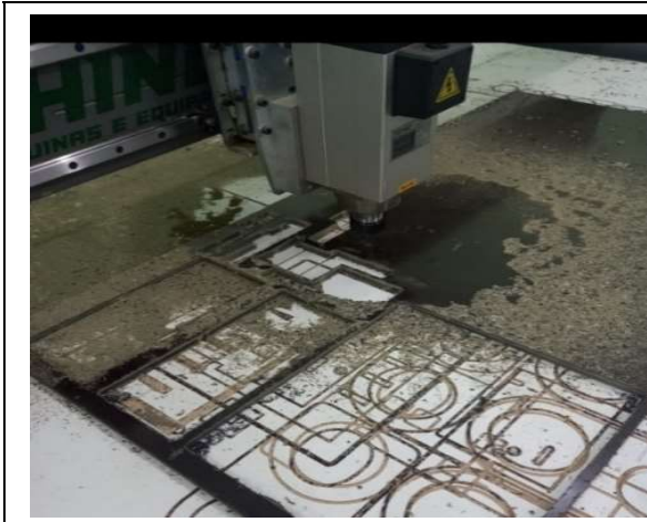
Figure 22. Machining the Upper Base
