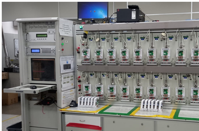
Figure 3. Benchmarking/adjustment of electronic meters
