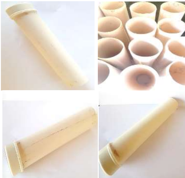
Figure 1. Molds used to cast specimens
