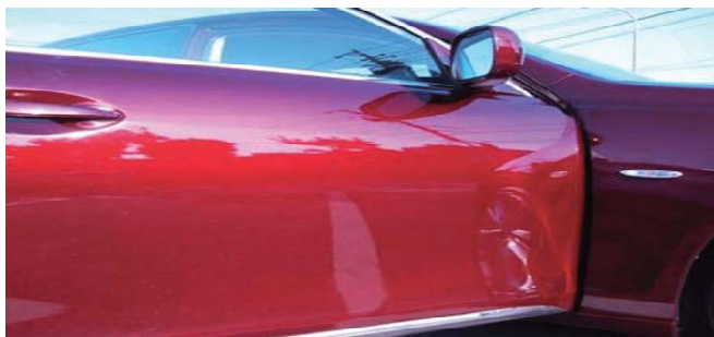
Figure 14. Photograph of a car to which was applied a clear coating containing gold nanoparticles on a red colored base coating.
