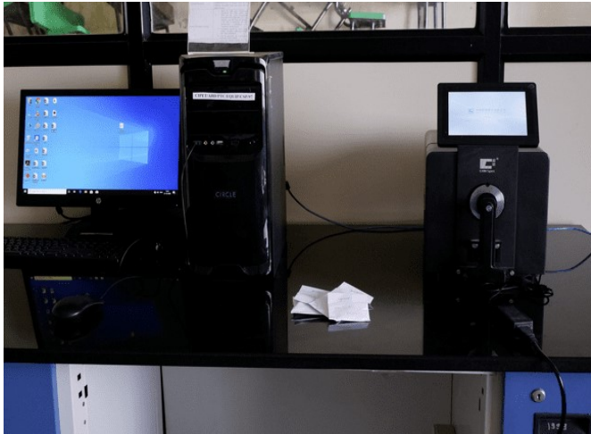
Armamentarium used for Evaluation of Translucency - spectrophotometer (Figure 4)
