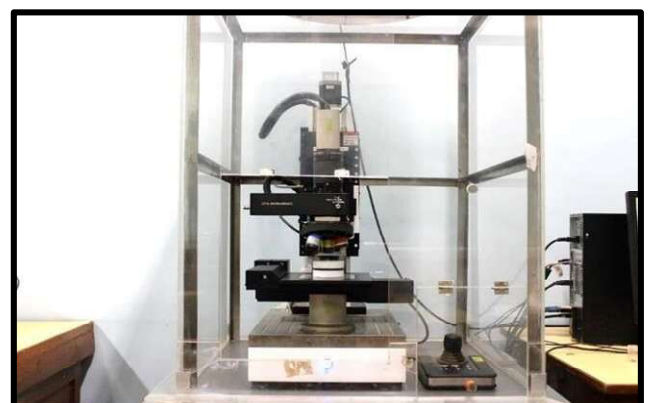
Armamentarium used for Evaluation of surface roughness-Profilometer (Figure 2)
