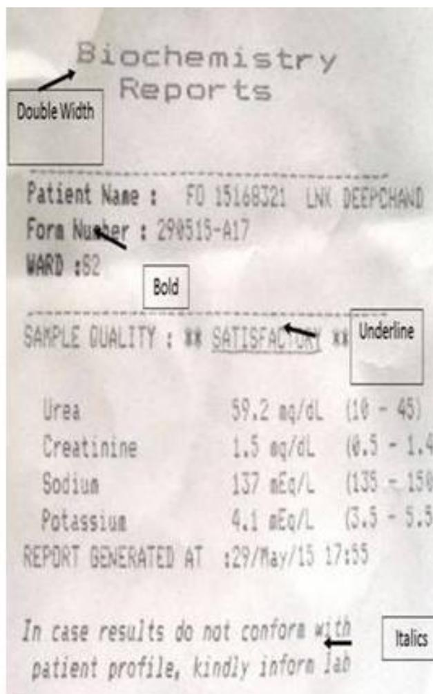
Figure 1. Examples of dot-matrix printer output using Esc/P codes
