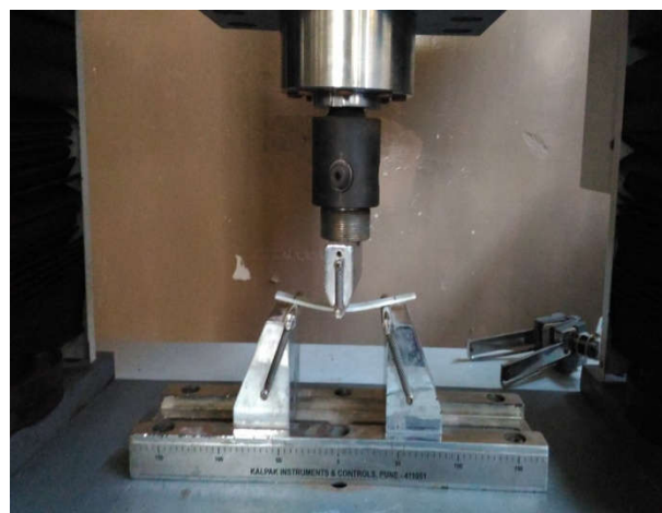
Fig. 4. Flexural testing setup
