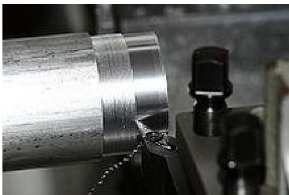
Fig. 1. Experimental setup Turning Process
