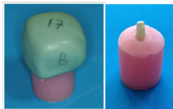
Fig. 3a. Silicon indexes for each specimen, Fig. 3b. Arrangement of the artificial gingiva
