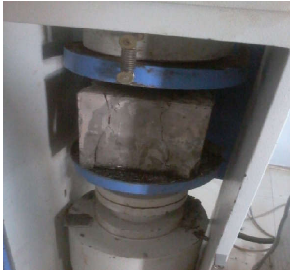
Fig 4. The compressive test and split tensile strength of concrete with fly ash and pumice
