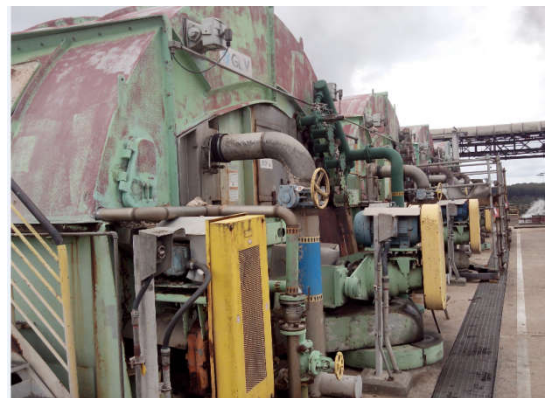
Figure 6. External detail of washer set
